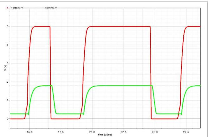
Figure 20. DDC/CEC Level Shifting Operation (B to A Direction)
