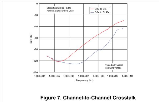
Figure 7. Channel-to-Channel Crosstalk
