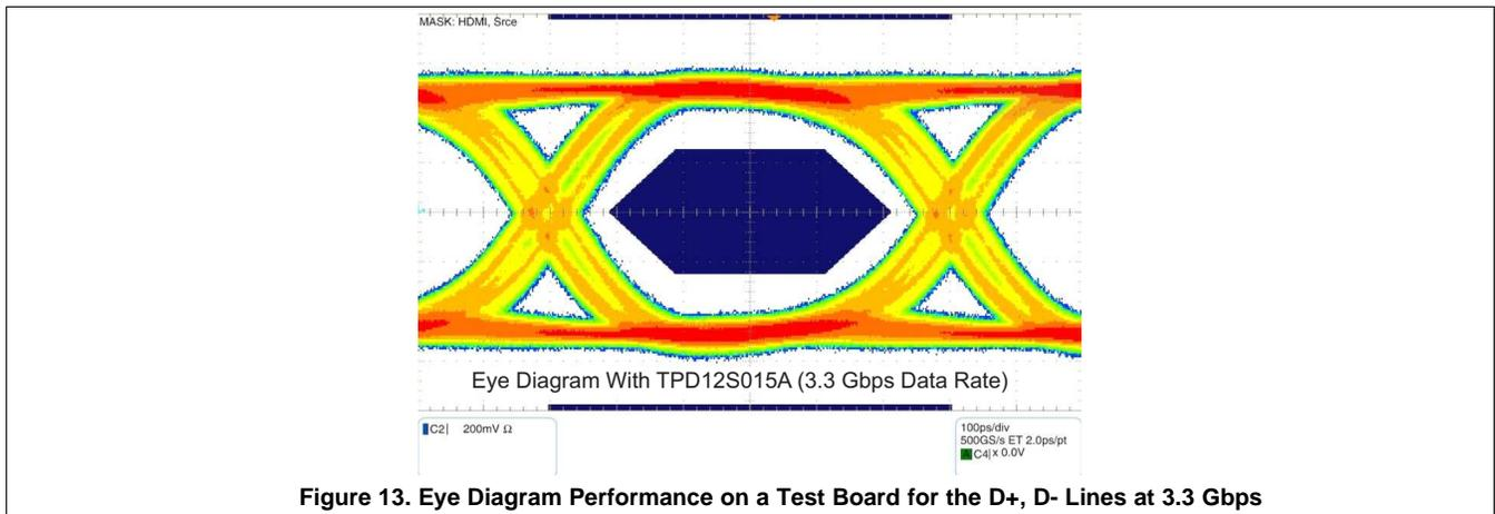
**Figure 13. Eye Diagram Performance on a Test Board for the D+, D- Lines at 3.3 Gbps**
