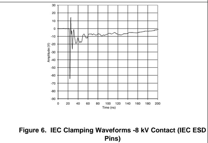
Figure 6. IEC Clamping Waveforms -8 kV Contact (IEC ESD Pins)
