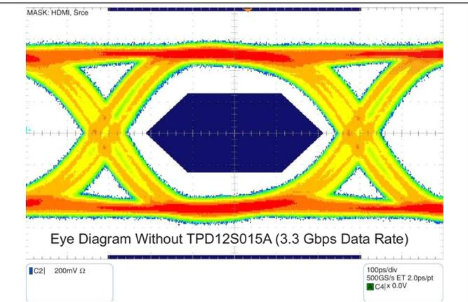
Figure 12. Eye Diagram Performance on a Test Board for the D+, D- Lines at 3.3 Gbps
