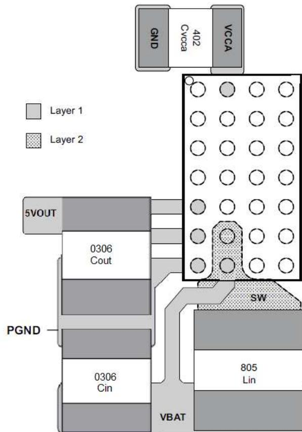
Figure 23. Board Layout (DC-DC Components) (Top View)
