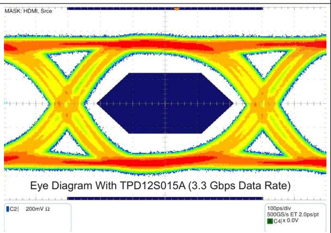
Figure 22. Eye Diagram Performance on a Test Board for the D+, D- Lines at 3.3 Gbps
