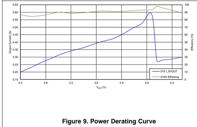
Figure 9. Power Derating Curve
