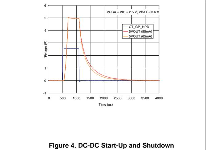
Figure 4. DC-DC Start-Up and Shutdown
