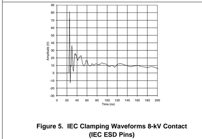
Figure 5. IEC Clamping Waveforms 8-kV Contact (IEC ESD Pins)
